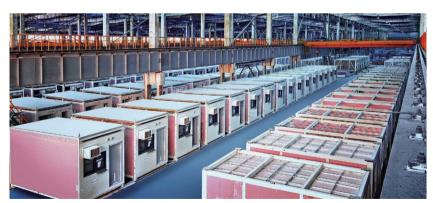
AluHouse provides users with MiC building solutions including development and production. Compared with the traditional on-site construction approach, MiC does not only minimize the duration of works on site, but also enhance productivity, site safety, environmental performance and sustainability.
