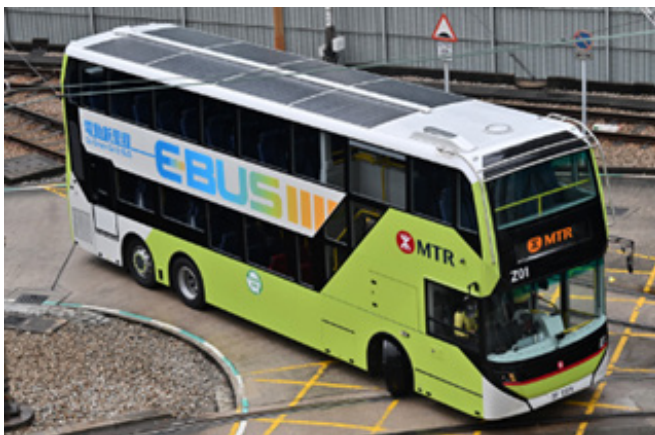
MTR's first electric bus is equipped with solar panels to power its ventilation system and LED lighting
