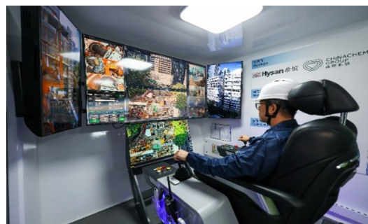
Remotely controlling the Distant Tower Crane Command System in a ground cabin
